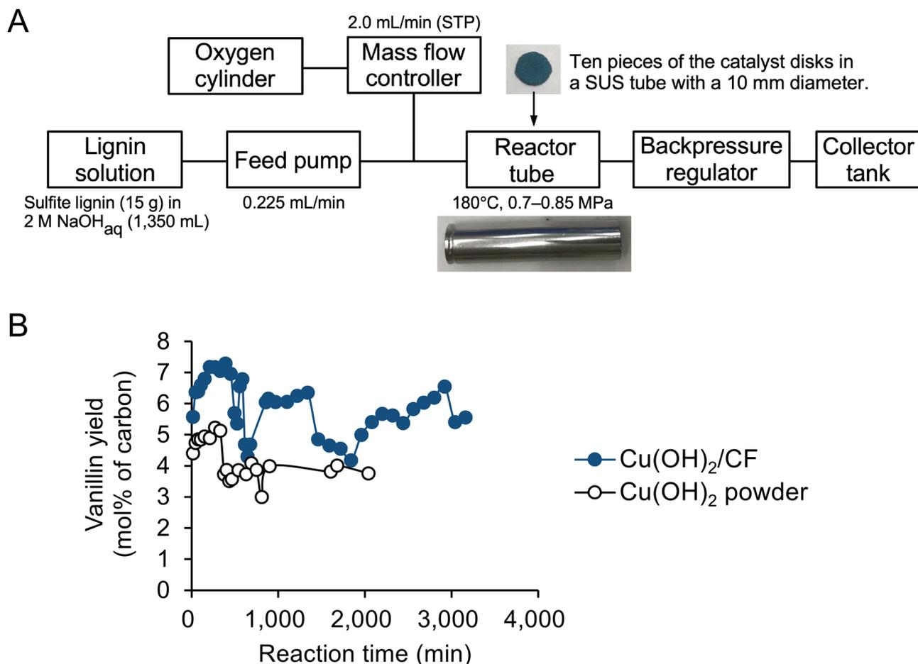
**Fig. 1** Outline of the Cu(OH)<sub>2</sub>/CF-packed column-equipped continuous flow reactor (**A**) and VN yield profiles (**B**). A single stainless column (10 mm in diameter, 50 mm in length) packed with 12 mmol of Cu<sup>2+</sup> carrying powdered Cu(OH)<sub>2</sub> (dot line, Tokyo Chemical Industry, Co. Ltd.) or Cu(OH)<sub>2</sub>/CF (solid line)
